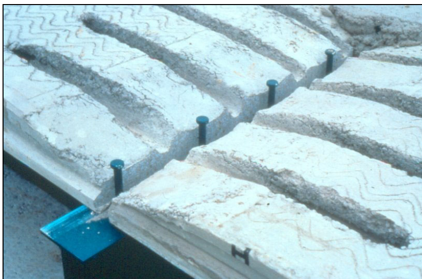
Figure 4.3 Composite beams supporting precast hollow-core units
