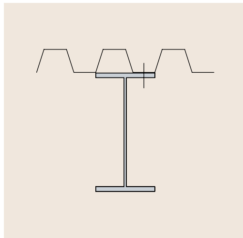
Figure 3.17 Decking spanning parallel to beam
