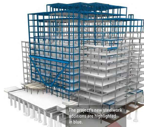
The western elevation is supported by raking columns and beams that connect back to the existing core.
