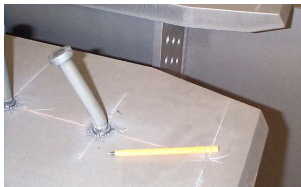
Figure 4 Shear stud after bend test
